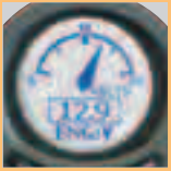
as a volt meter for single engine
